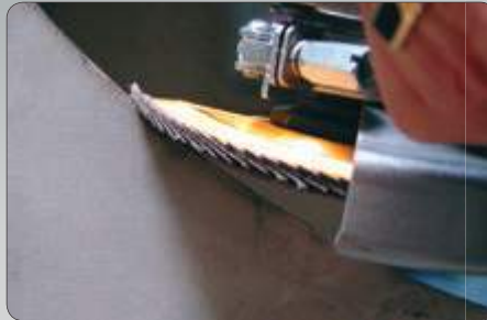
Large contact area due to high elasticity.
