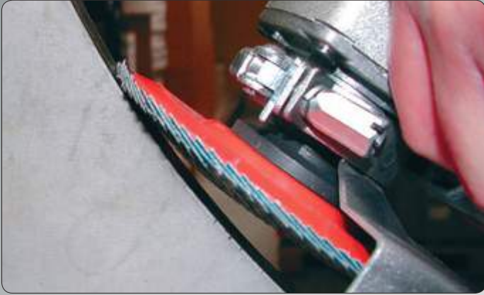
Large contact area due to high elasticity.
