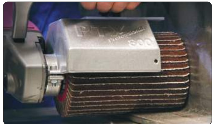
The overhang on 150 mm wide rollers means that you can work in the internal edges with ease.
