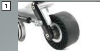
1 The new damping system with gas pressure dampers.
