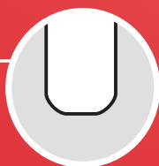
Deburring both sides of the sheet edges. Does not change the sheet dimensions.
