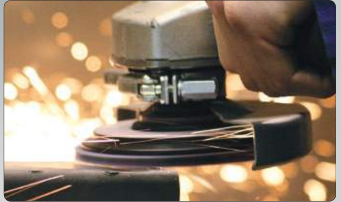
Flat support surface for perfect weld transitions on external edges. Ideal for tank and control cabinet manufacturing.
