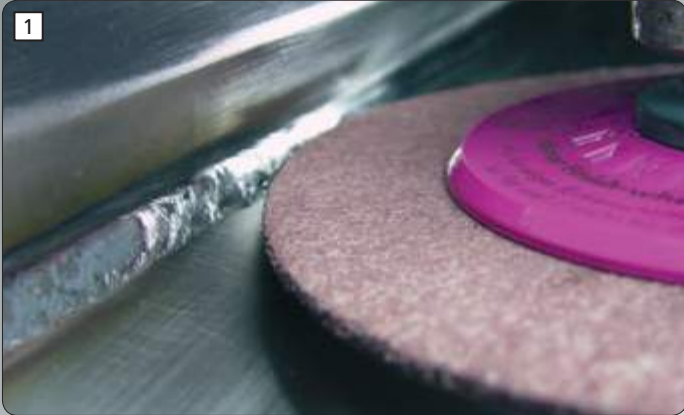
1 Pre-grind and level finer welds with the red POLY MAGIC WHEEL, grit A (80).
