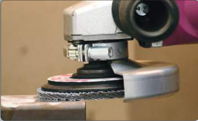
Flat support surface for perfect weld transitions on external edges. Ideal for tank and control cabinet manufacturing.
