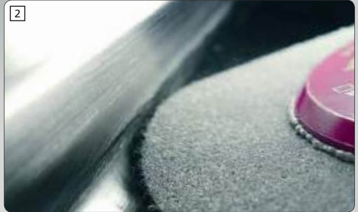
2 Polishing to an impeccable mirror finish using the grey POLY MAGIC WHEEL, grit B (900).
