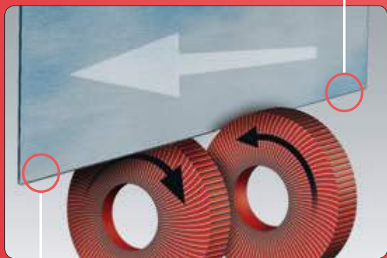
Sheet with burr after cutting
