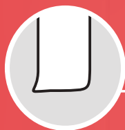
Sheet with burr after cutting
